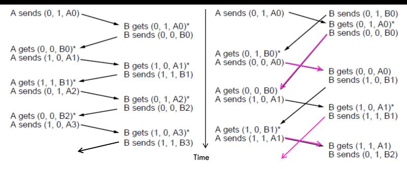
Notation is (seq, ack, frame number). Asterisk indicates frame accepted by network layer .
